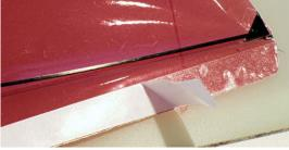
**H.** Fold over the 'flaps' along the dashed line on the template, the 'fold line'. And press and rub to bond the double sided tape to the backside of the flap and to the back side of the skin.
